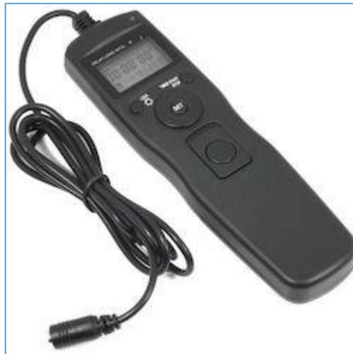
I prefer the wired release because you are always near the camera to make adjustments etc. and therefore within the range of the connecting cable. It also has a big advantage of having a built-in timer that allows for interval shots and also timed release. A tip for the remote is to fix some Velcro on the back of it and have the other portion on the tripod and easily holds the timer handy. The Infra Red remote is good to set up the camera and take selfies etc.
