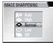
The example at left is from a Nikon camera and is typical of JPEG controls. You have "Auto", Low, Normal, High or Off. The only way to see which setting suits your purpose is to do some experiments to see what works best for you with your camera. This is obviously a fairly blunt tool.
